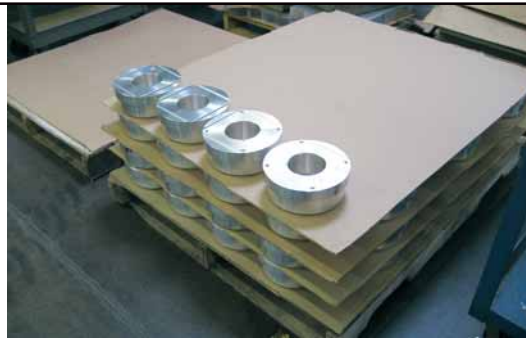
The SV1 main bodies are made from a single chunk of high quality aluminum. Here you see a pallet of partially machined billets waiting to go on to the next step in becoming the worlds baddest carbs. RIGHT - Here we have some finished mains, ready to be assembled. One of them could be on its way to adorn a competitors bullet.
