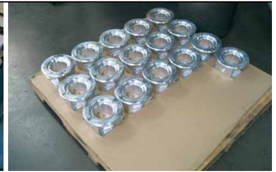
The SV1 main bodies are made from a single chunk of high quality aluminum. Here you see a pallet of partially machined billets waiting to go on to the next step in becoming the worlds baddest carbs. RIGHT - Here we have some finished mains, ready to be assembled. One of them could be on its way to adorn a competitors bullet.
